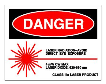
b) Aperture Safety Label. This label is located inside the engraver's cabinet, at the right rear, above the aperture through which the engraving laser and Laser Diode Pointer beams enter the cabinet.
